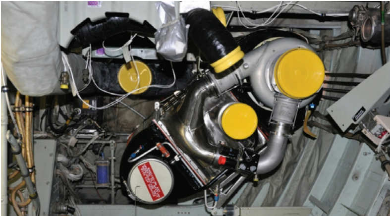
New ECS Refrigeration Unit
